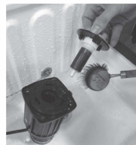
4. Take rotor out and clean with water and brush
